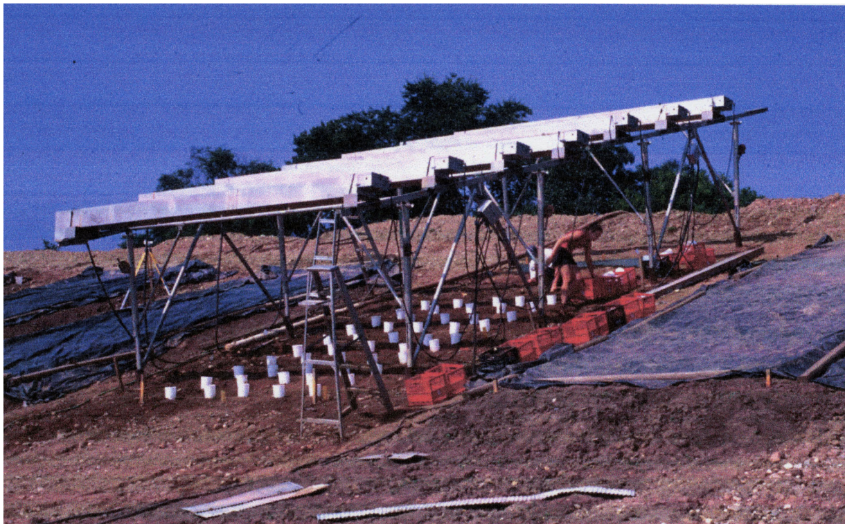
Figure 1. Programmable rainfall simulator used in the field experiment set up for testing and calibration.
