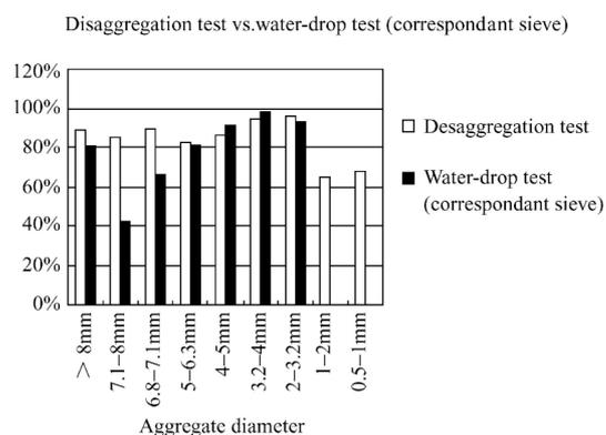
**Fig.1** Disaggregation test and water-drop test
