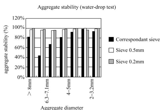
**Fig.2** Aggregate stability (water-drop test)
