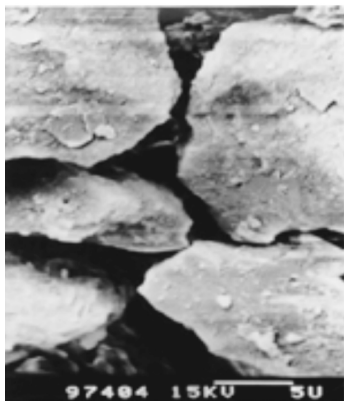
Fig.1 SEM micrograph of structural crust. Original magnification (O.M.) 3500×
