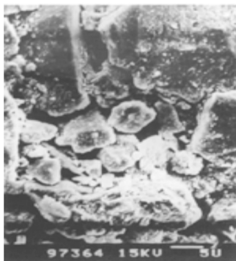
Fig.3 SEM micrograph of depositional crust. (O.M.) 2000×
