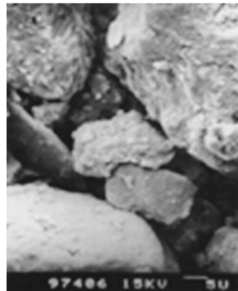
Fig.2 SEM micrograph of depositional crust. (O.M.) 1500×
