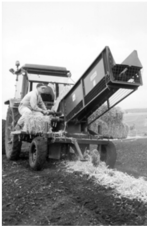
Fig.2 Laying straw mulch on rip lines in a recently sown onion crop
