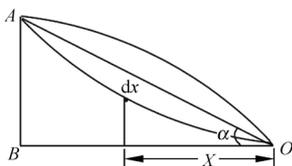
Fig. 2 Expression of even slope, concave slope and convex slope
