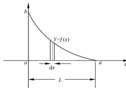
Fig. 3 Calculating chart of runoff energy to concave slope
