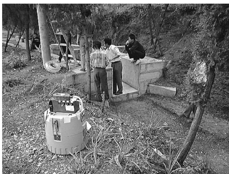
Fig. 4 Installation of a sampler at a flume
