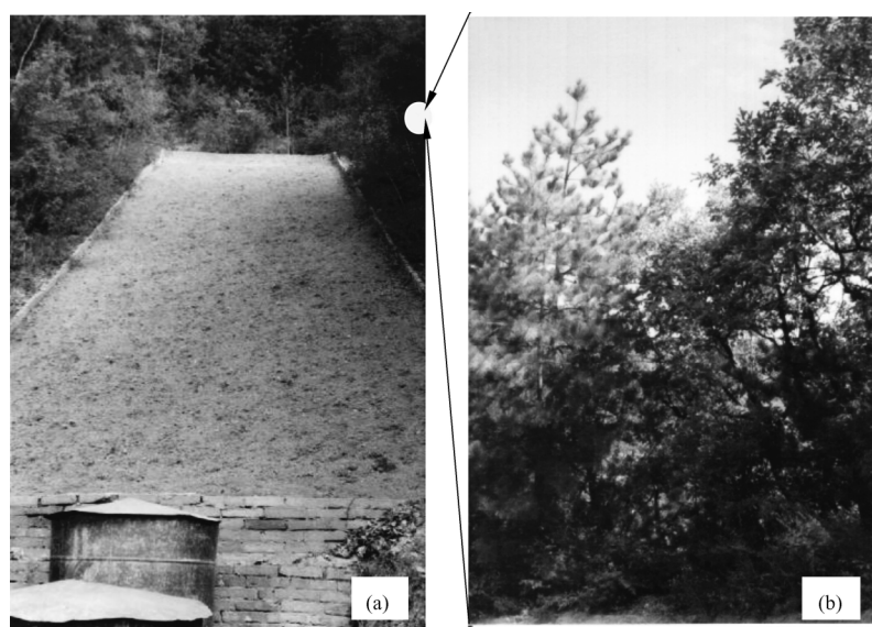
Fig. 1 Natural runoff plots for monitoring the influence of cultivation on soil properties with concern of soil erosion. (a) cultivated fallow land plot with area of 995.2 m 2 and average slope degree of 26° ; (b) natural forest plot with area of 965.8 m 2 and average degree of 24.3°, the main vegetation species are Q. liaotungensis , P. tabulaeformis Carr., P. davidiana , B. platyphyllum , S. viciifolia , O. davidiana , Z. guguba , A. gmelinii , and P. betulaefolia Bge
