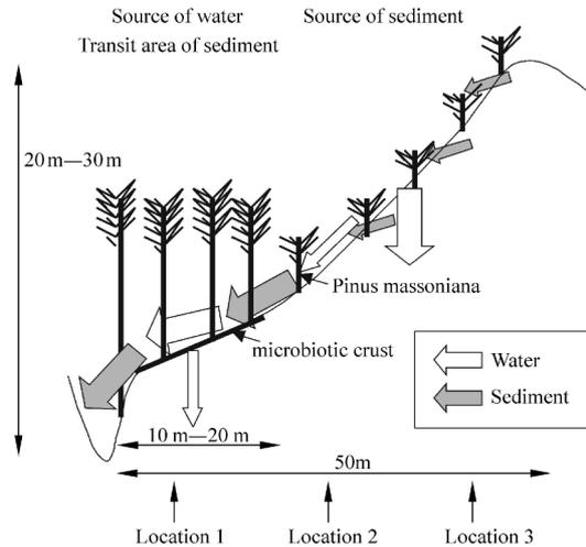
**Fig. 1** Schematic illustration describing the mechanism of the sediment production and transport in Dahou Experimental watershed
