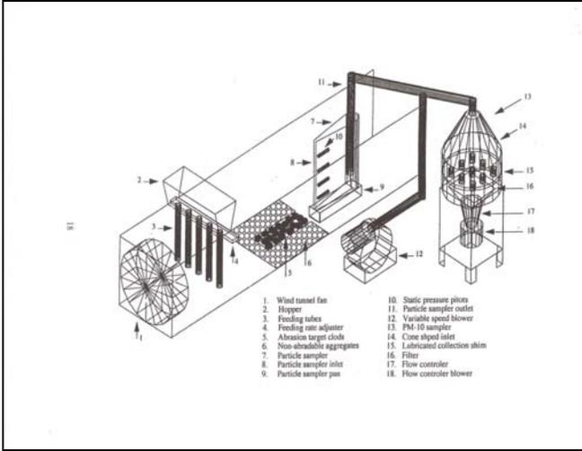
Figure 2. Diagram of wind tunnel and sampling equipment used for clod abrasion tests.
