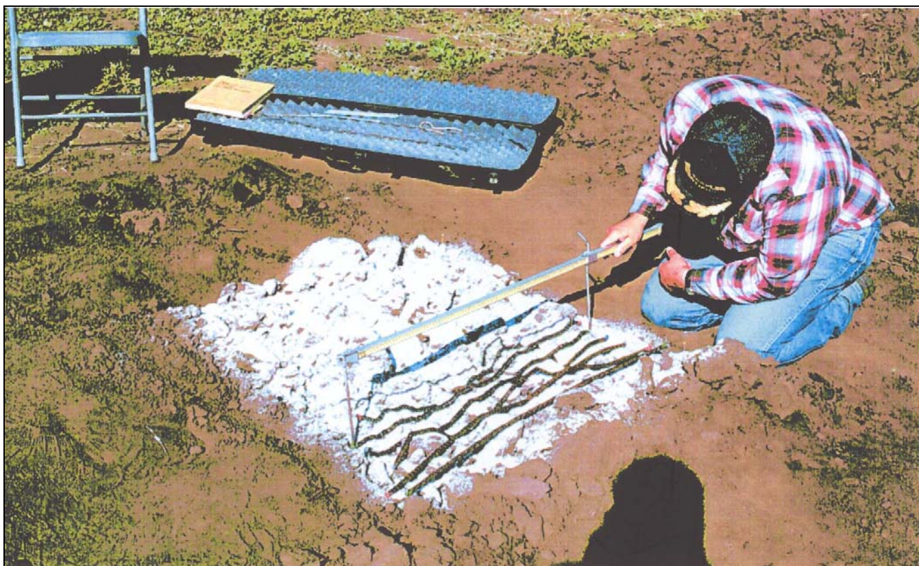
Figure 3. Illustrating chain set measurements being conducted in the field.
