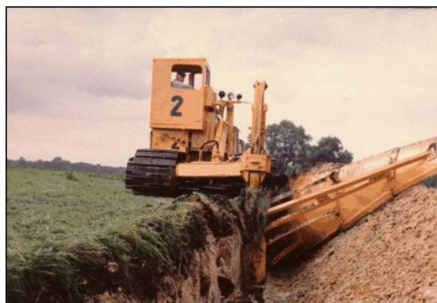
Figure 2. Plowing with 3 or 4 caterpillars -500 kW - up to 2 m depth as depending on Histosol thickness. Middle-granular sand in underground, groundwater level between 0.8 and 1.3 m below the surface.
