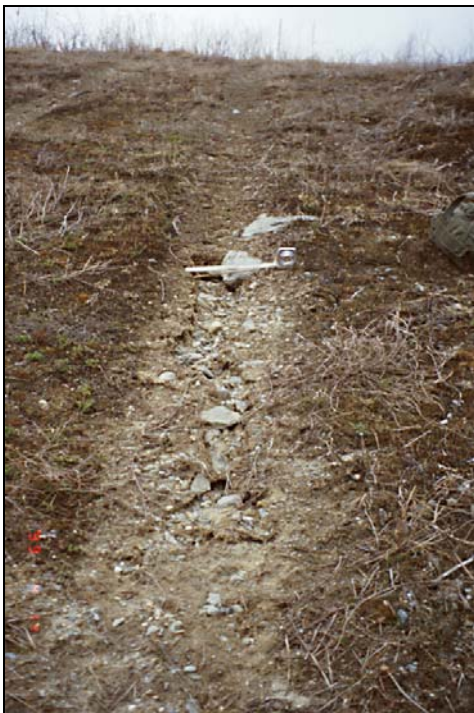
Figure 7. Rills formed over the 1998-99 winter in HEMTT ruts (W1) in vehicle plot #4, which has a 31% (17°) slope; (a Top) south rut with 1- to 2-cm-deep rills scattered along its length, (b Bottom) north rut with a 7- to 10-cm-deep rill in the mid-slope part of the rut, note the tape measure for scale. Photographs taken on 14 April 1999.
