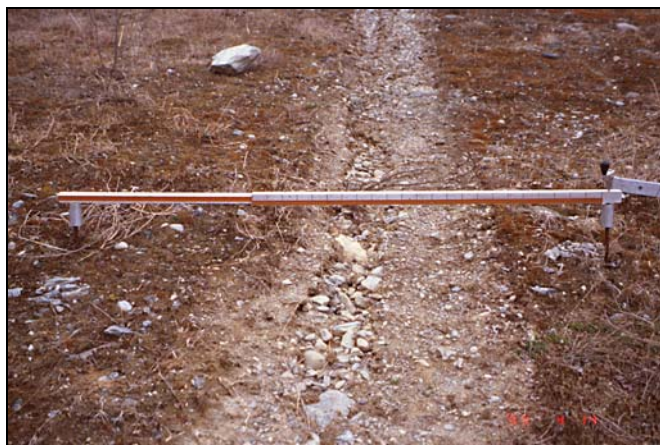
Figure 3. Rebar-mounted bar used as datum for measuring rut and rill cross sections. Note the 7-cm-deep rill under the bar on this 14 April 1999 photograph. The rill formed over the 1998-99 winter in the mid-slope part of the south rut of tank rut 2 (T2) in vehicle plot #3, which has a 31% (17°) slope (see Figure 2).
