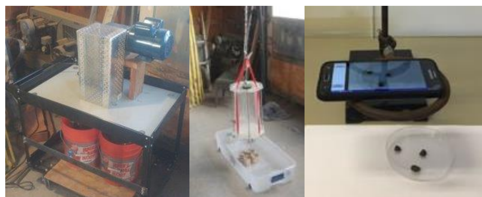
Fig. 1. Methods used for aggregate stability included wet sieving (left), Cornell Sprinkle Infiltrometer (middle), and the Slakes phone application (right) (data not presented here).
