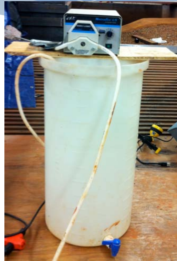
Flocculant injection system
