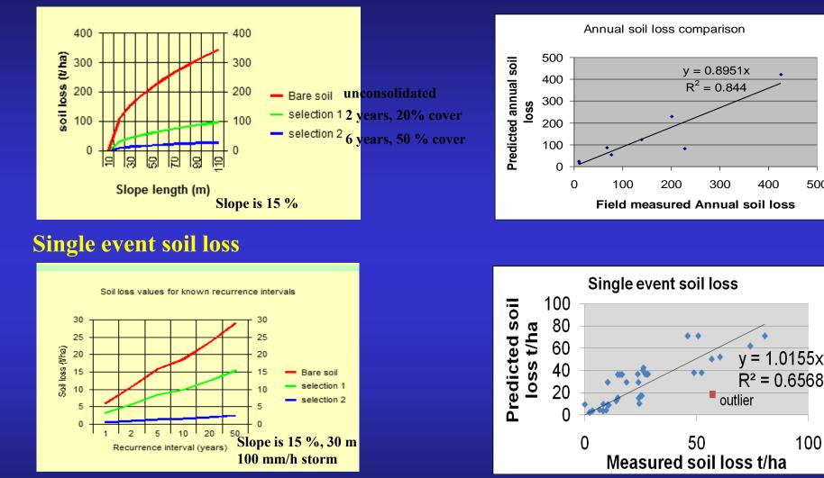
**Although MINErosion 3 can be used to derive suitable combinations of slope** length and gradient, it cannot be used to assess erosion from landscapes. Need to combine it with GIS to assess erosion from catchments/landscapes.
