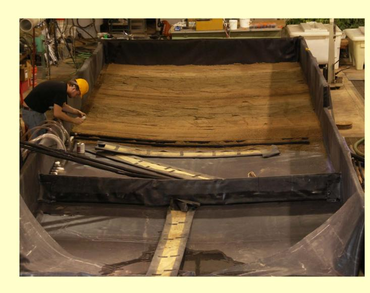
Water table control pipes in sand layer
