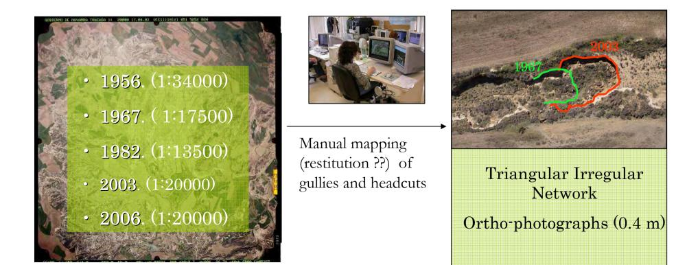
Using the DEMs and the ortho-photographs, volumetric headcut retreat rates for each period were calculated as the product of the lineal retreat and a representative sectional area of the headcut.
